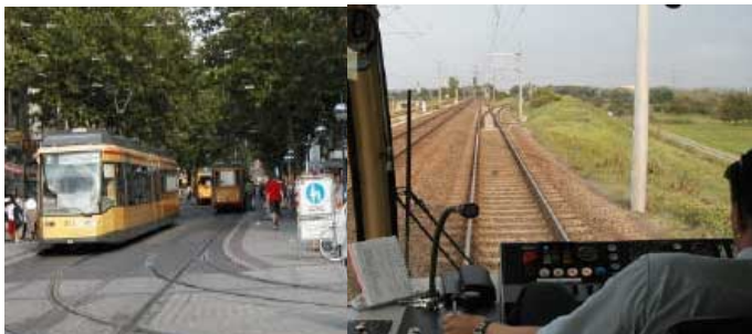
Dual-mode trams can run on both streets and heavy rail lines
